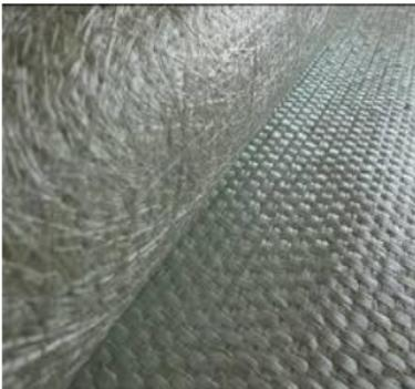
Figure 1. Bidirectional and woven fiber (Mallick, 2007).<sup>9</sup>
