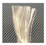
Figure 2. Unidirectional fiber (Mallick, 2007).9
